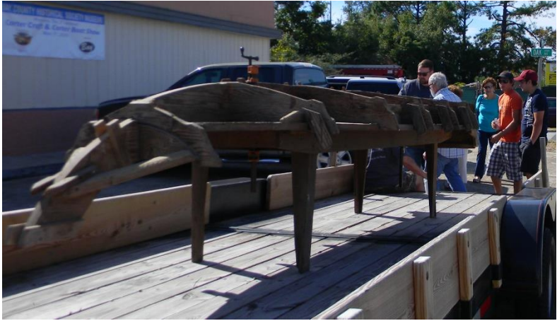
Frame for making 12 and 14 ft Carter Boats Provided by Harlan Wilson
